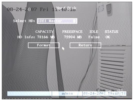
fig 6.5 Hard Disk setup
